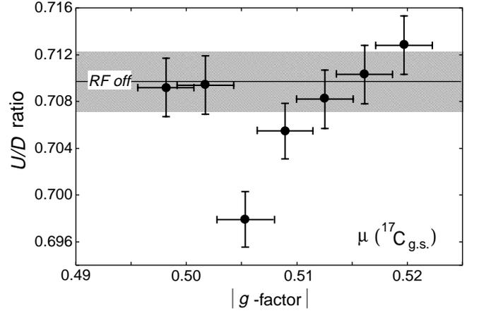
**Fig. 4.**  $\beta$ -NMR spectrum obtained in the measurement of the  $g$ -factor of  $^{17}\text{C}$ , with bin widths ( $\Delta\nu/\nu$ ) of 0.01.
