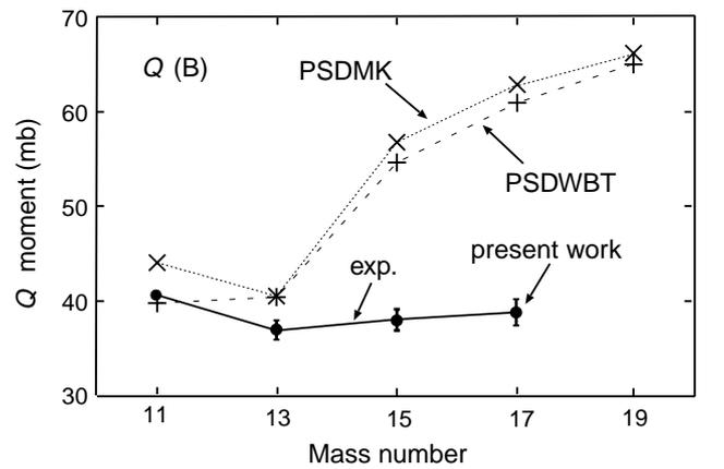
**Fig. 5.** Comparison between the experimental (exp.) and theoretical  $Q$  moments for odd-mass B isotopes. The calculated  $Q$  moments, using the effective interactions PSDMK and PSDWBT with  $e_p = 1.3$  and  $e_n = 0.5$ , increase with the mass number in the neutron-rich region, while the experimental values are almost stable against the mass number and are considerably smaller than the shell model calculations for  $A = 15$  and  $A = 17$ .
